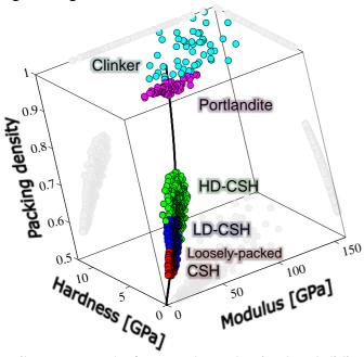
In situ assessment of cement mechanics by statistical cluster analysis of nanoindentation properties for a portland cement. Colors represent different mechanical phases in the hardened cement paste, with low (LD) and high-density (HD) CSH being dominant by volume fraction. Hardness and modulus measurements relate to strength and elastic properties, respectively.
